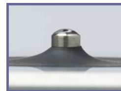
Un-conditioned Pedestal- water “Flattens out”
