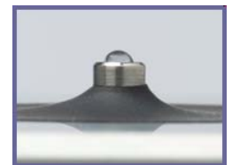
Properly Conditioned Pedestal-water “Beads up”
